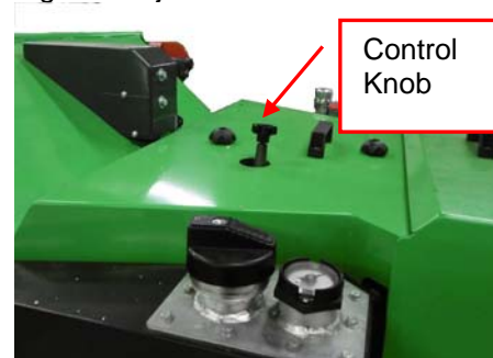
Fig 5.8 Adjustable feed roller control
