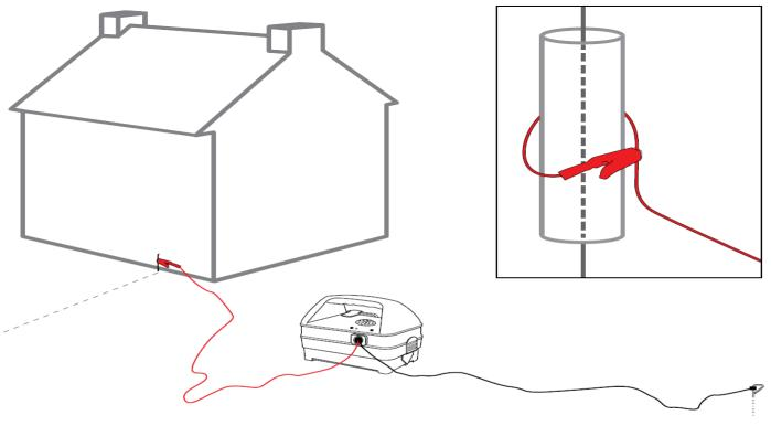
Signal jumping from an accessible cable
