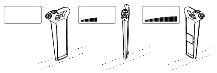
Trace the buried conductor keeping the C.A.T4 vertical and moving it steadily from side to side. Follow the line of the buried conductor, marking it as required across the area to be excavated.
