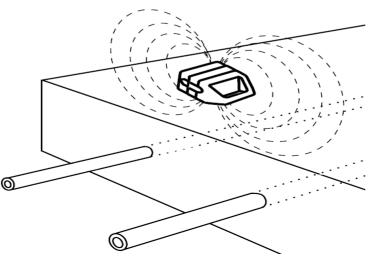
Estimating line depth using the C.A.T4+/eC.A.T4+ and Genny4
