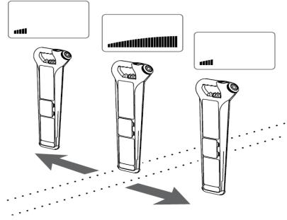
and forth across the maximum readout position, the cable or pipe's position can be pinpointed. The tidemark feature hold the maximum bargraph reading to ease identification of a peak readout.
