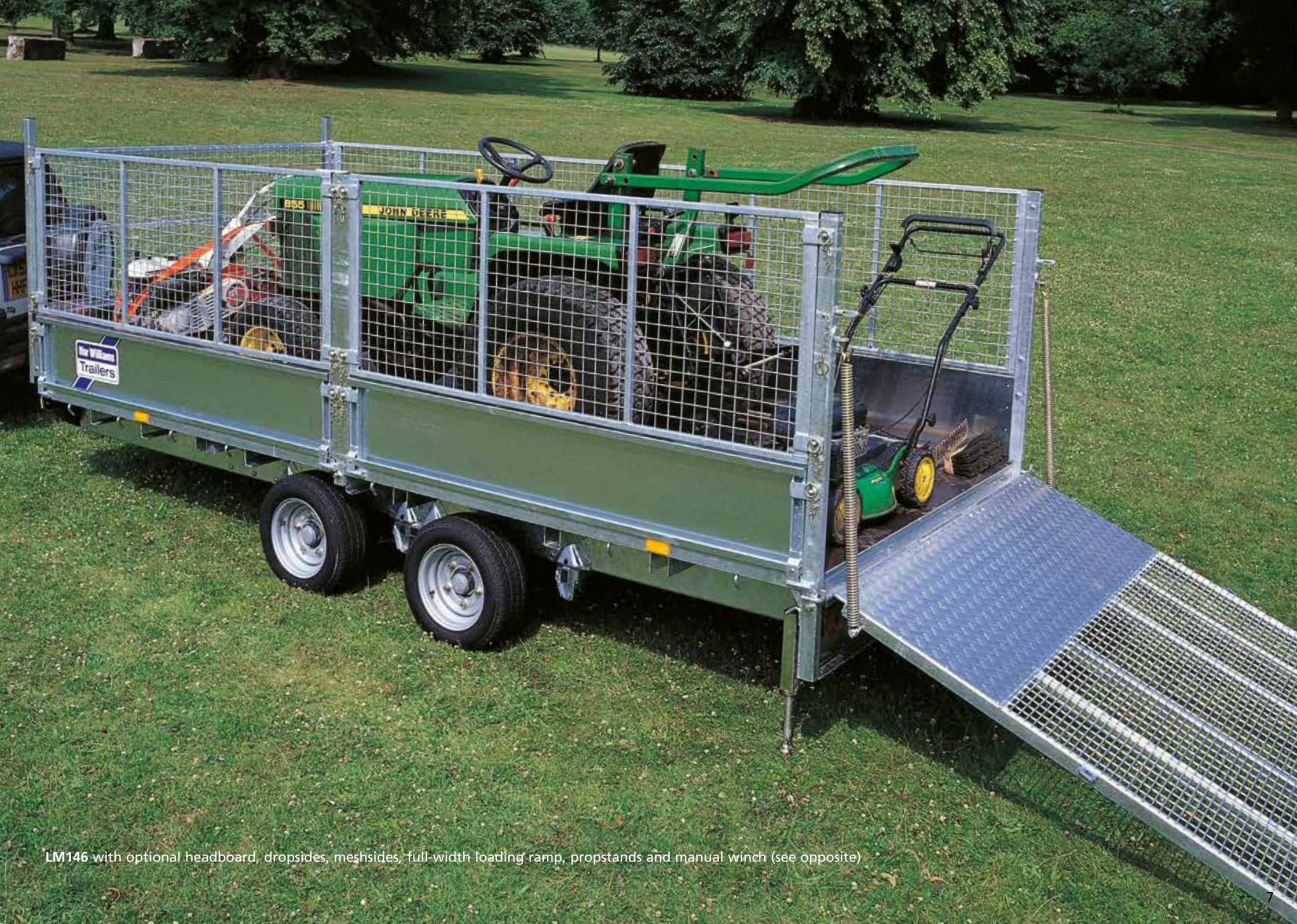
LM146 with optional headboard, dropsides, meshsides, full-width loading ramp, propstands and manual winch (see opposite)
