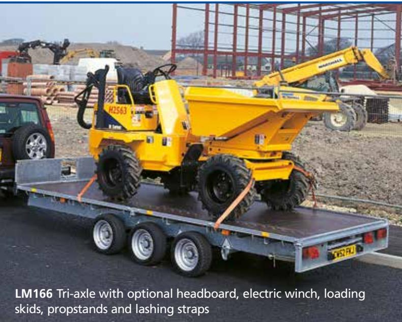
LM166 Tri-axle with optional headboard, electric winch, loading skids, propstands and lashing straps
