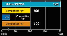
Blade used for tests: 185mm (7-1/4") TCT saw blade (24T) supplied with Makita 5007MG Test material: 2x10" (38x230mm) SPF timber
