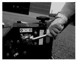
The Ground Drive Clutch Lever effects the front wheels only. Pull the lever back and down to the stop to engage ground drive. Up and forward is neutral or free wheel.
