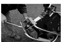
Tilt the machine forward and rest onto the front frame.
