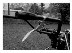
The Throttle Lever increases the engine speed to engage drive.
