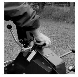
Turn the Depth-Set Dial to the required depth observing the depth scale, which is calibrated 0-8 cm (0-3").
