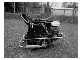
The Operators Handles fold for storage or carriage.
