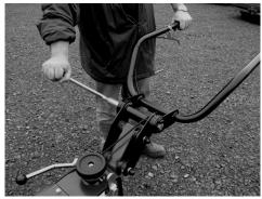
To adjust Operators Handles loosen locking lever and adjust to a comfortable working height. Re-clamp the lever firmly.
