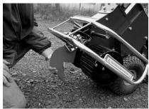
To fit Mole-Drain or Decompaction Blades locate the blade studs into crossbar, fit and tighten the nuts. The Heavy Washers are not required.
