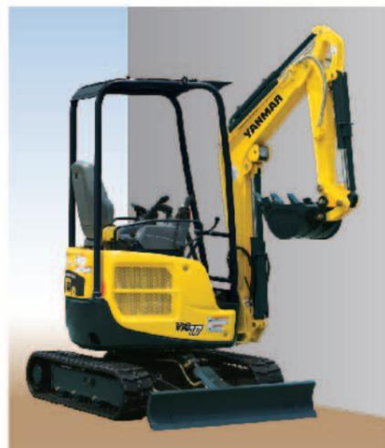
Side Ditch Digging up to the Wall without Sticking Out beyond the Track.
